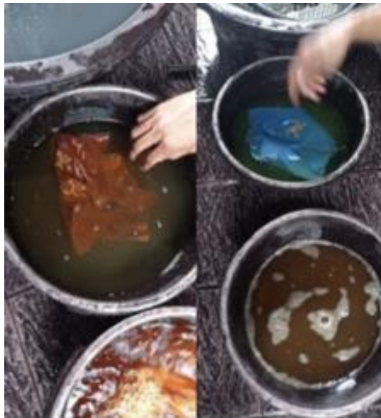
Fig 13. The fabric with a solution of naphthol dye
