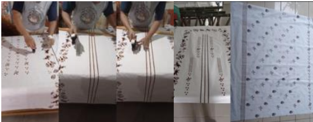
Fig 17. The stamping process
