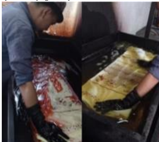
Fig 18. The staining process in the naphethanol liquid
