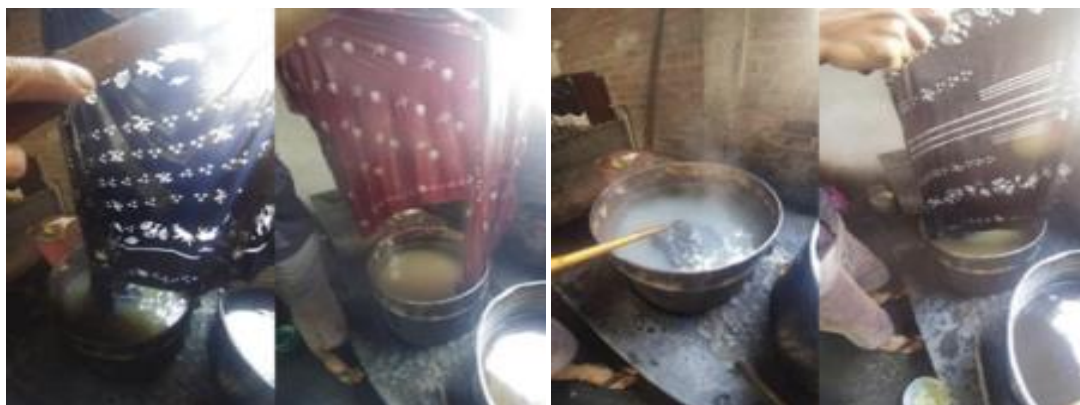
Fig 20. The process of loosening or softening wax on the fabric
