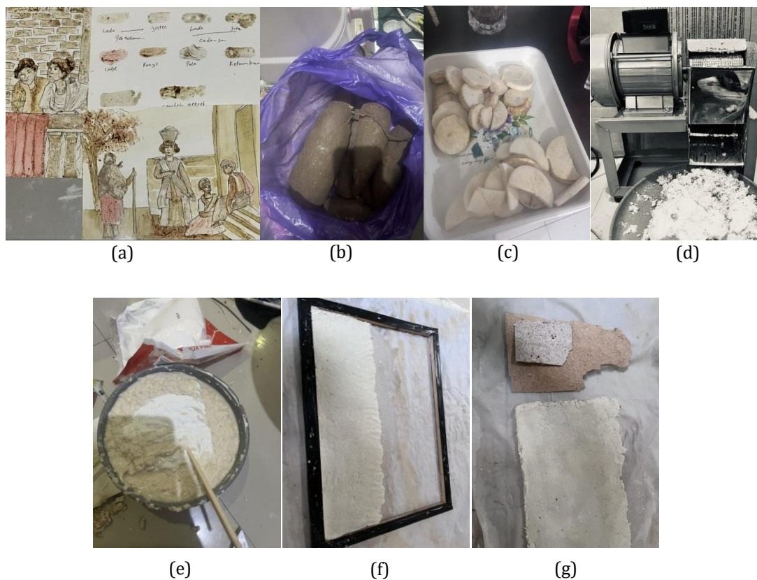
Fig 12. (a) Natural dye application on watercolor paper; (b–g) stages of cassava-based art paper production from tuber preparation to A4 sheet finishing.
