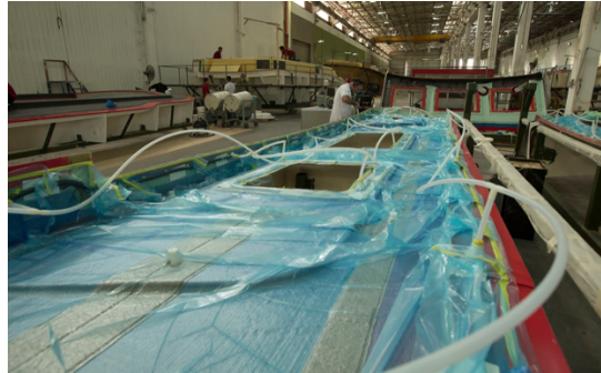
Figure 3. The hull of the new Grand Banks is made of a conventional layup of vacuum.
